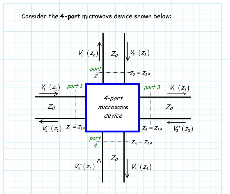
Note in this example, there are four **identical** transmission lines connected to the same "box". Inside this box there may be a very **simple** linear device/circuit, **or** it might contain a very large and **complex** linear microwave system.
