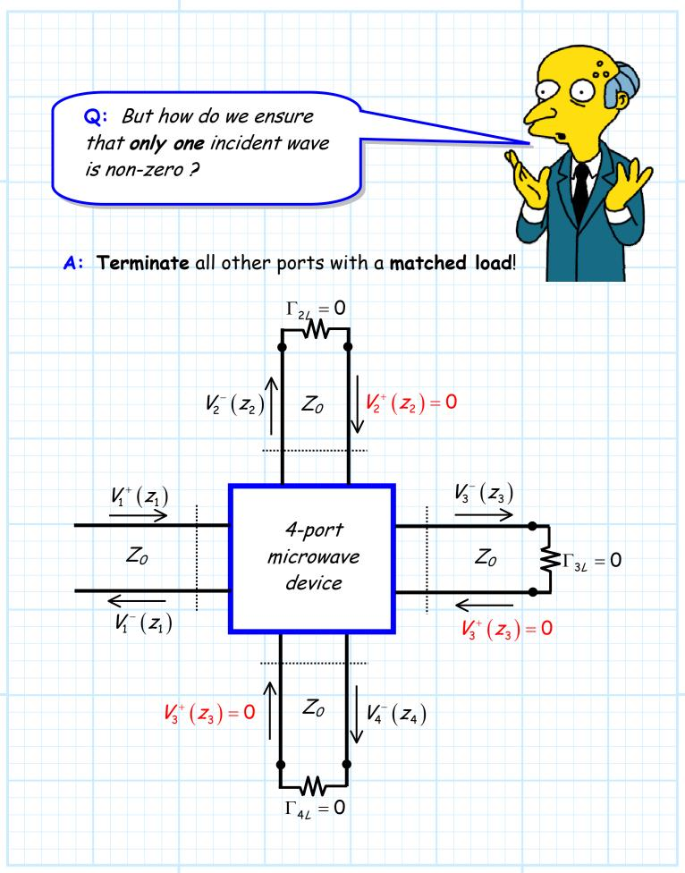
Note that if the ports are terminated in a matched load (i.e.,  $Z_L = Z_0$ ), then  $\Gamma_{nL} = 0$  and therefore:
